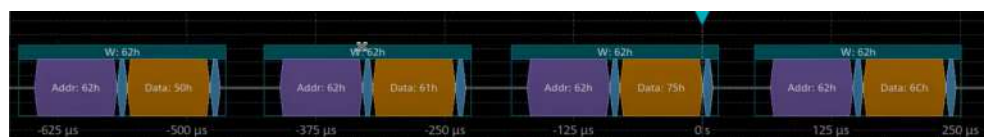
Figure 14-15: Trigger on Type=Data, Data=0x75 and Position=1
