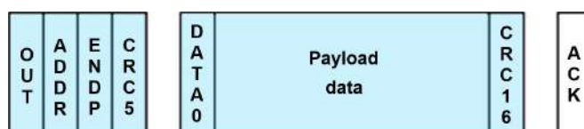
Figure 14-55: Example of a bulk OUT transfer. Blue: host speaks, white: device speaks
