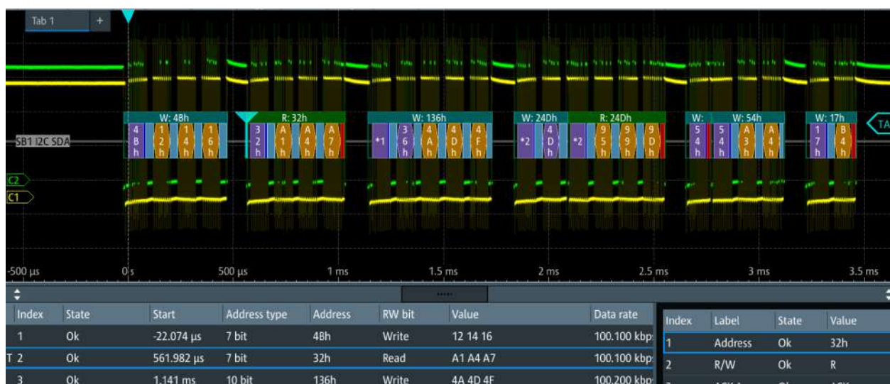
Figure 14-6: Example of sequence trigger in I2C signal with "Trigger A" (interval > 1 ms) and software trigger (first "Read" frame)
